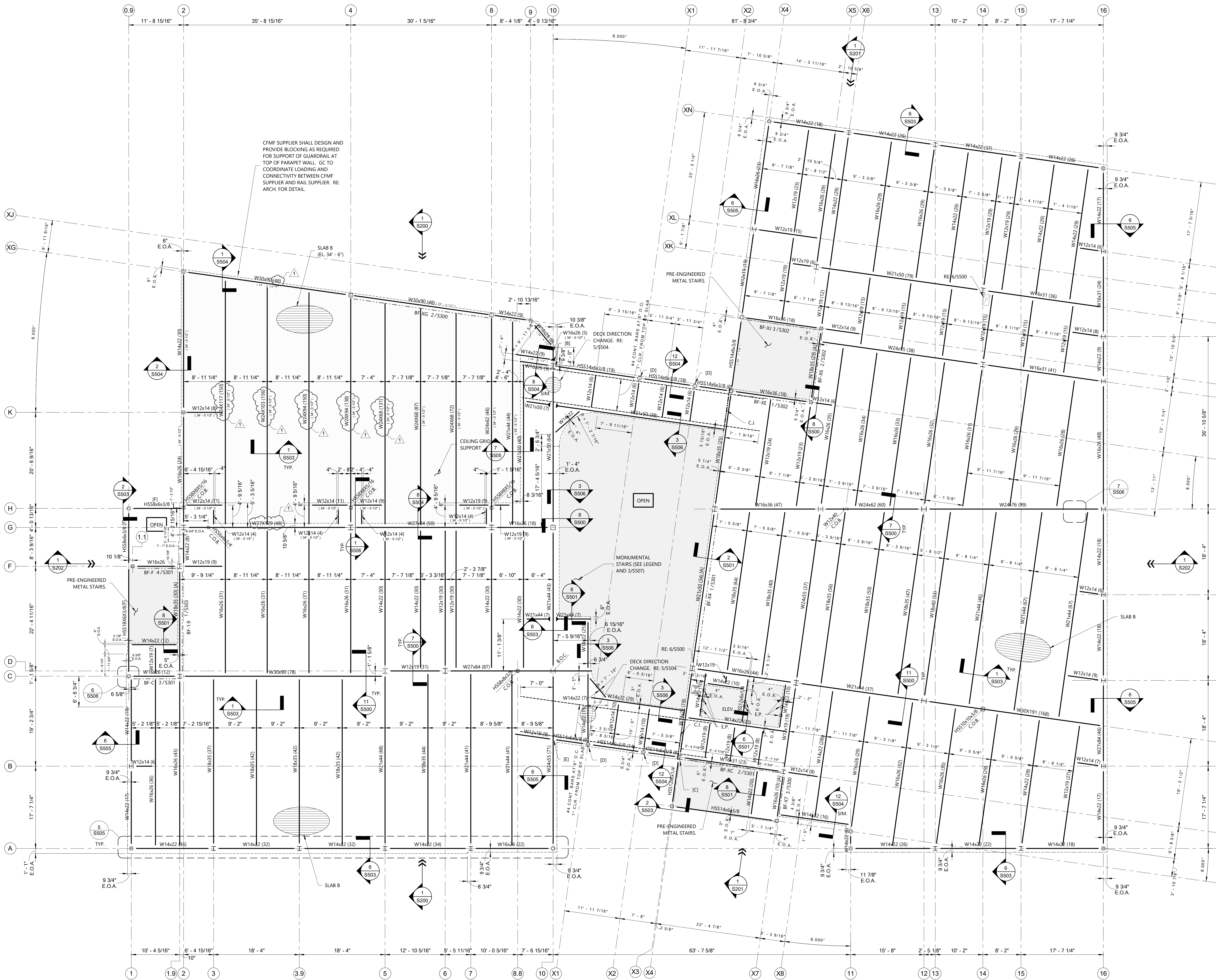
1 THIRD FLOOR FRAMING PLAN 1/8" = 1'-0" (T.O.S. AT EL. 35'-2 1/2" U.N.O.)
